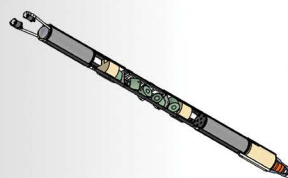
ROVOPI Small Pipeline Inspection
